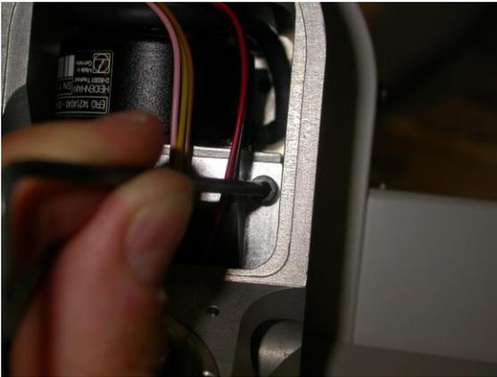
4. Note the positioning of the cabling in the assembly as this will be crucial to re-assembling the motor.
